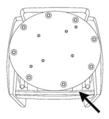
Step 2 Attach the enclosed Rechargeable Battery Pack using its 'Snap-On' system with the pre-installed mounting plastic bracket.
